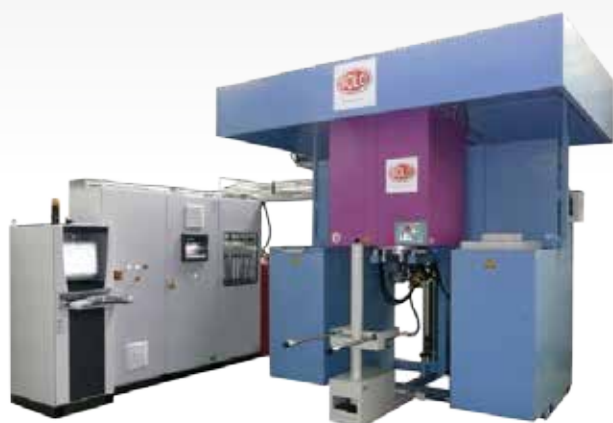
1 furnace and 2 tanks
